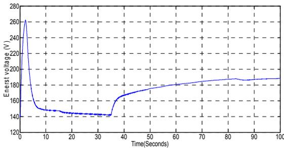
**Fig.16:** Enerst voltage of the fuel cell.
