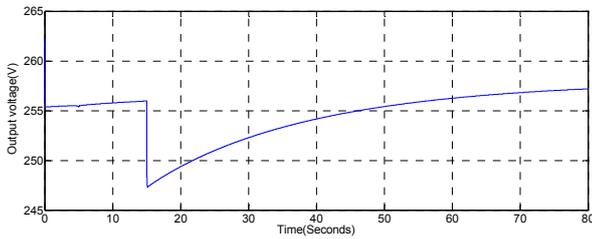
**Fig. 9:** Output voltage of the fuel cell.
