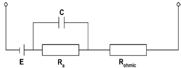
**Fig.4:** FC electrical equivalent circuit
