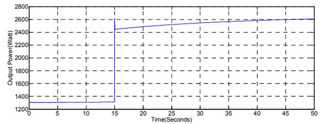
**Fig. 7:** Output power of the fuel cell.
