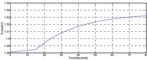
**Fig. 10:** Enerst of each cell of the fuel cell
