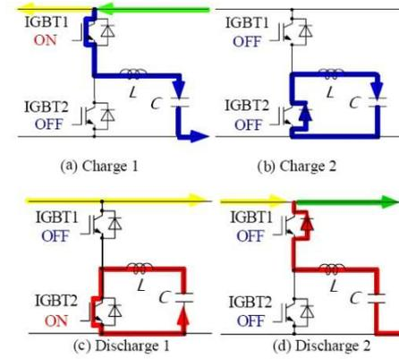
**Fig. 6:** Operation of the circuit in charge and discharge modes [7].
