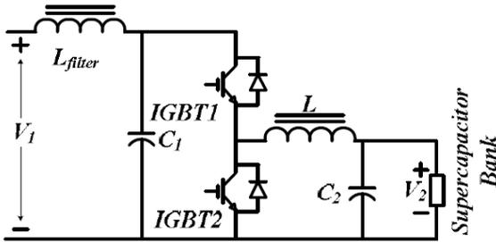
**Fig. 5:** Bidirectional buck-boost converter used in this work [7].
