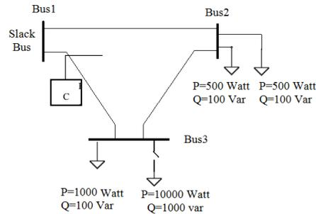
**Fig.14:** Distribution system used in simulations.
