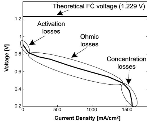
**Fig.3:** Typical FC polarization curve [6].
