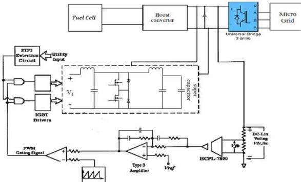
**Fig.2:** The configuration of the control system.
