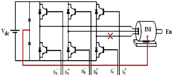
**Fig. 5:** Scheme of the inverter for faulty machine
