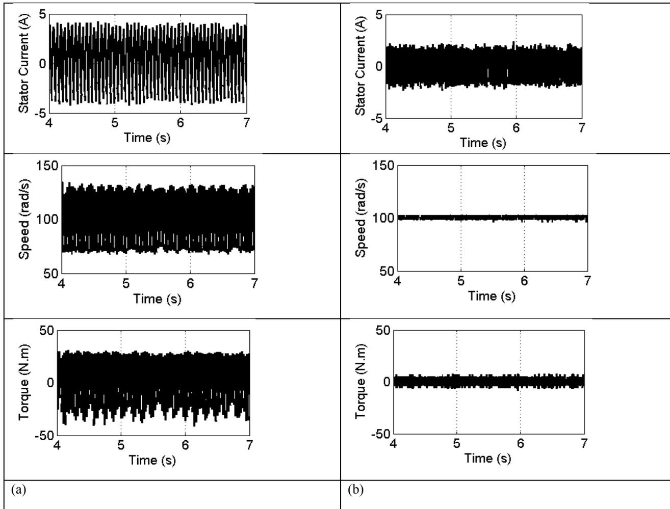
**Fig. 6:** Simulation results of the conventional and proposed method for vector control of the faulty machine; (a): Conventional method, (b) Proposed method
