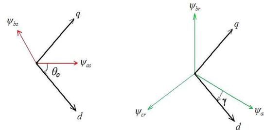
**Fig. 2:** Stator and rotor winding's flux axes
