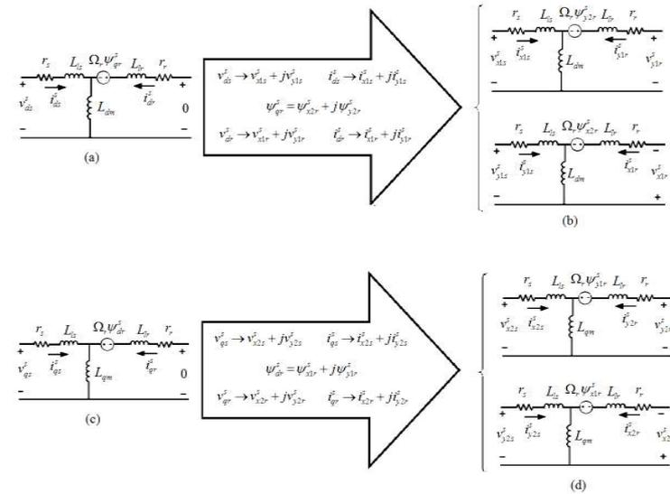
**Fig. 3:** Equivalent circuit of the 3-phase IM under open-phase fault
