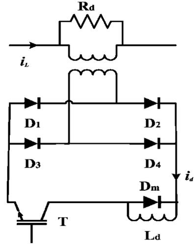
Fig. 1. RBFCL power circuit
