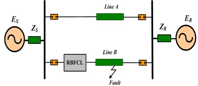
**Fig. 2.** The test system
