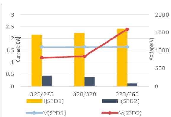
**Fig. 5:** Discharge voltages and currents of the SPDs
