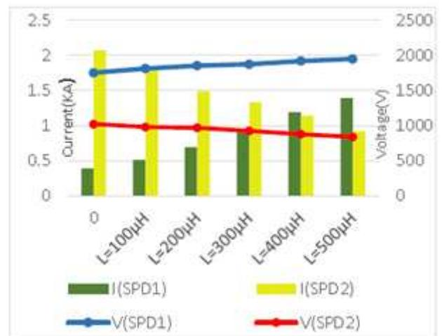
Fig. 12: Variations of the discharges' voltages and currents vs. different values of the inductive impedance
