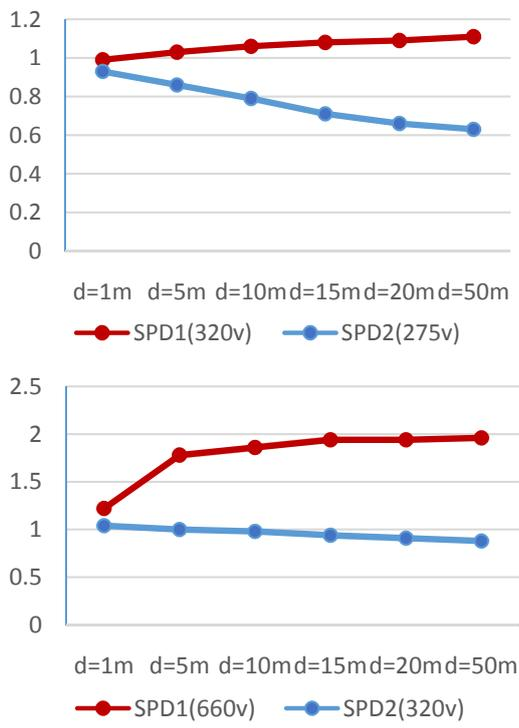
Fig. 11: Voltages of SPDs vs the variations of distance between them
