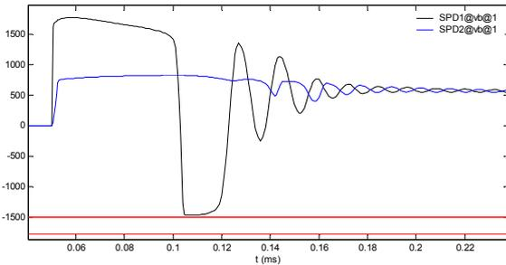
Fig. 8: the voltage’s waveforms of the SPDs;SPD1:660V- SPD2:320V
