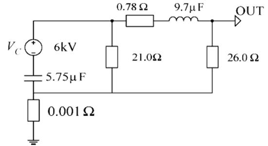
Fig. 2: The simulator circuit of voltage and current of lightning waves
