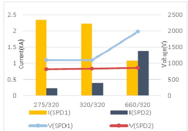
**Fig. 6:** Discharge voltages and currents of the SPDs (SPD2:SPD320v)
