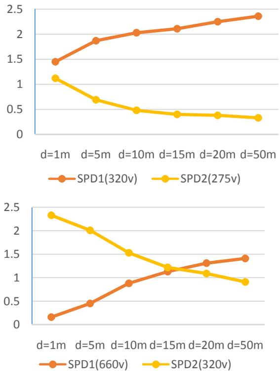
Fig. 10: The discharged currents of protection SPDs against variation of the cable length from 1m to 50m
