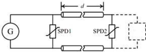
**Fig.4:** The single phase low voltage network under study
