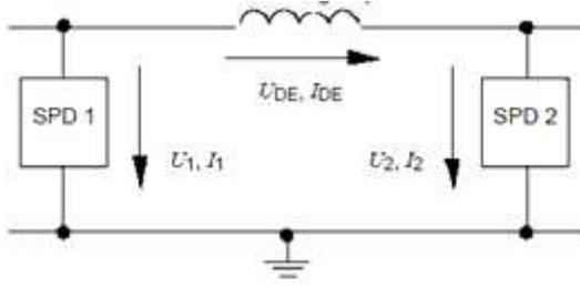
Fig 1: Using the inductance in order to coordinate the two SPDs [1]
