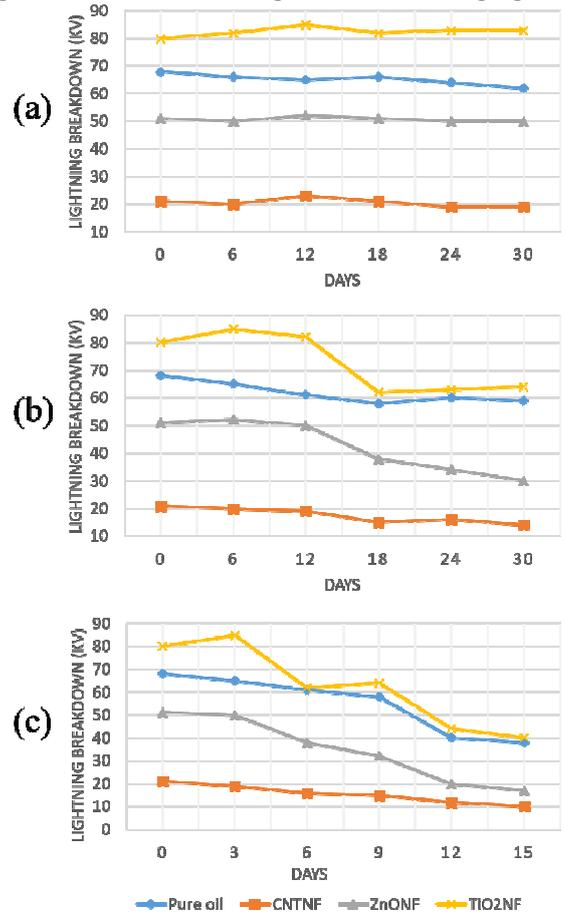
**Figure3:** The results of lightning breakdown voltage tests for (a)110°C; (b)120°C; and (c) 130°C
