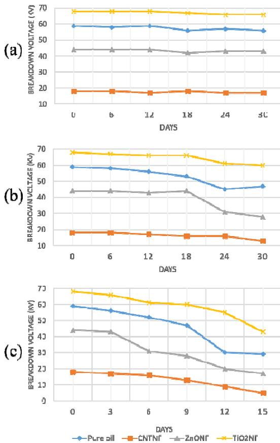
**Figure2:** The results of breakdown voltage tests for (a)110°C; (b)120°C; and (c) 130°C
