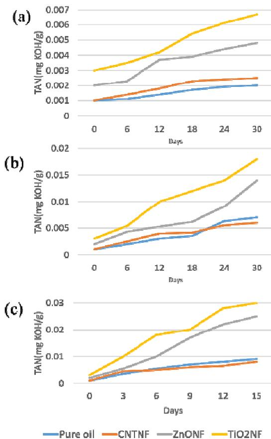
**Figure 1:** The results of TAN test for (a)110°C; (b)120°C; and (c) 130°C
