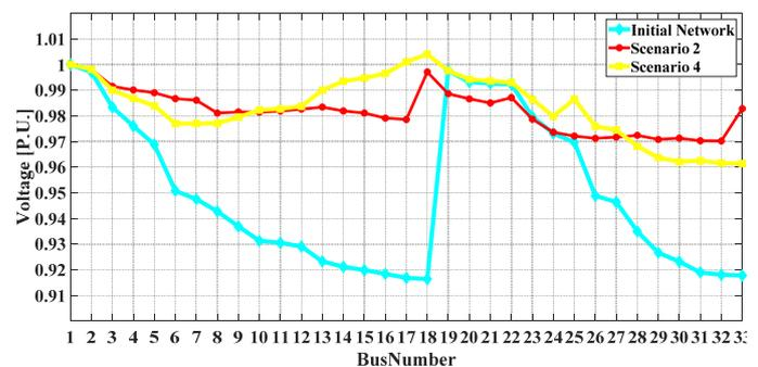
**Figure 4:** Voltage profile for network buses at hour 19
