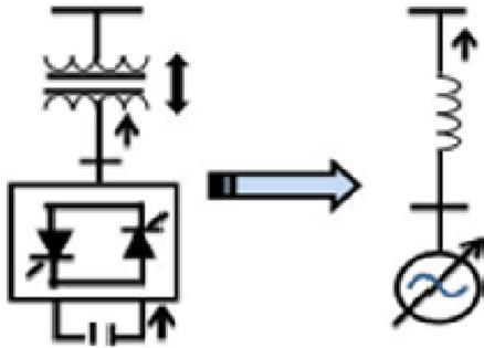
Figure 1: Structure of Static synchronous compensator (STATCOM)
