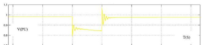
Figure 9. Voltage domain characteristic of wind farm bus with 3MW
