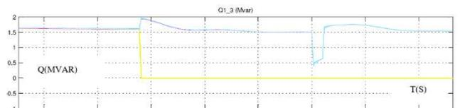
Figure 7. Output of reactive power –wind turbine
