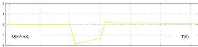
**Figure 10.** Output of reactive power in connected network with 3MW STATCOM
