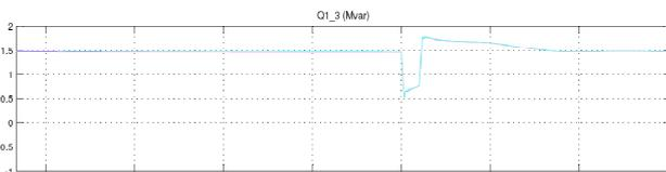
**Figure 12.** Output of reactive power –wind turbine
